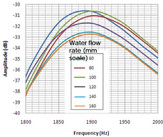
Figure 8 : Amplitude responses for the frequency of 1,900 Hz on the varied water flow rates.
