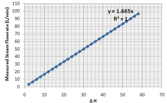
Figure 11 : Result of calibration for steam flow rates.
