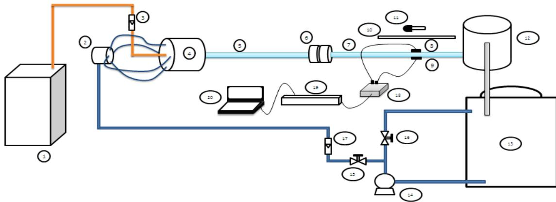
Figure 1: The pipe installation and the equipment and apparatus arrangement for experiment.
