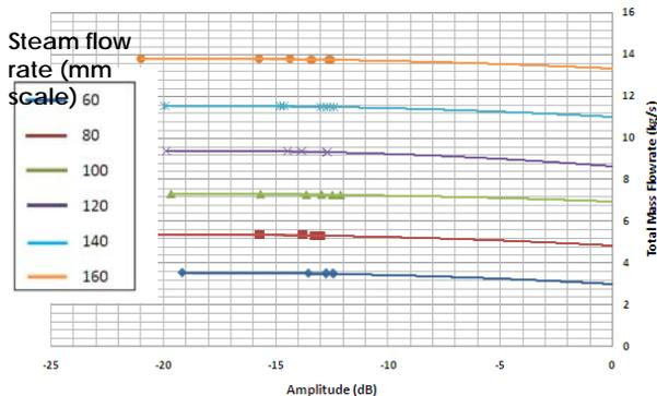
Figure 12 : The correlation between total mass flow rate vs RMS amplitude for various steam rate at the frequency of 1,900 Hz.
