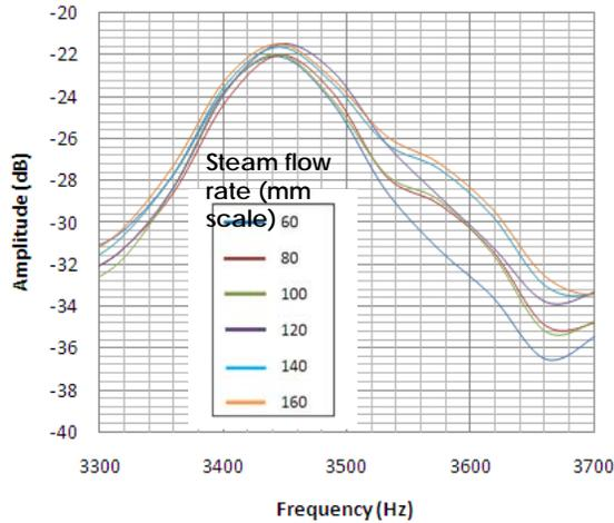
Figure 7 : Amplitude responses for the frequency of 3,500 Hz on the varied steam flow rates.
