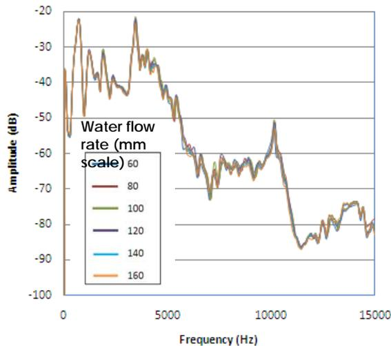
Figure 4 : Amplitude responses with the frequencies due to white noise signal on the varied water flow rates.
