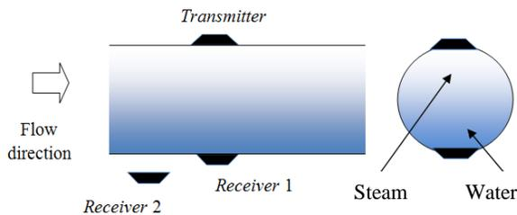
Figure 3: The transducer mounting.
