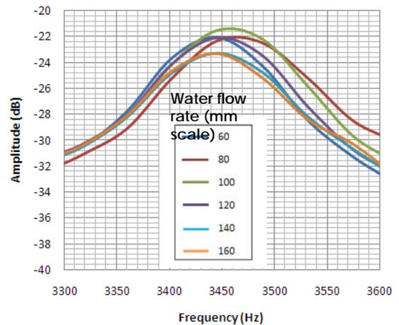
Figure 6 : Amplitude responses for the frequency of 3,500 Hz on the varied water flow rates.
