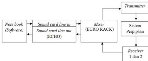
Figure 2: Block diagram of the hardware.
