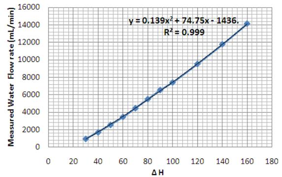
Figure 10 : Result of calibration for water flow rates.
