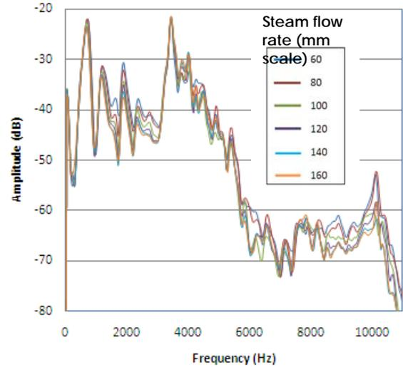
Figure 5 : Amplitude responses with the frequencies due to white noise signal on the varied steam flow rates.
