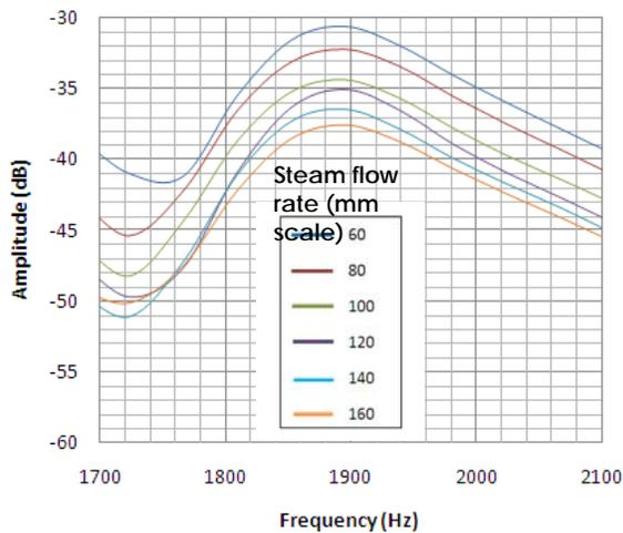
Figure 9 : Amplitude responses for the frequency of 1,900 Hz on the varied steam flow rates.
