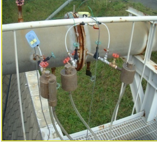
Figure 2: Arrangement of Devices in Orifice Flow Meter.
